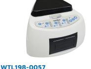
MiniBio Auto reader Compact design, Allows incubating 3 indicators simultaneously, in different incubation times, at the same temperature.
